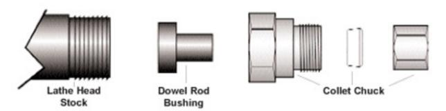
Designed for 3/8" hardwood dowel rods, this chuck is inexpensive and effective for turning toy tops and bottle. The chuck screws directly onto your 3/4" 16 TPI headstock. With the collet chuck, you receive the dowel rod bushing. Stock #1100-A.
